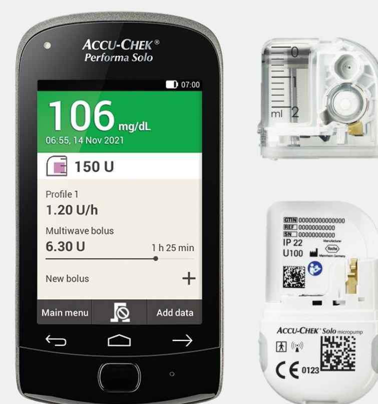
Figure 1: The Accu-Chek® Solo micropump system. The modular micropump system is either controlled remotely via the diabetes manager (shown on the left side) or allows bolusing directly on the pump (shown on the right side). Due to the modular design including a reusable pump base (lower part) and disposables (upper part) the components can be replaced independently from each other. For a better comprehensiveness, the components of the pump are illustrated disassembled. A more detailed description of the system can be found in (1).
